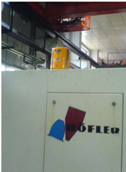
NASA 42T installation on CNC machine Note: Due to space constraint, the cylinder stays outside the panel while the automatic discharge nozzle goes inside the panel
